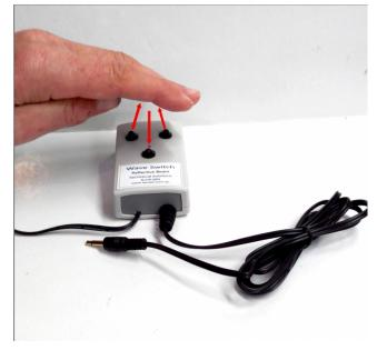
An infrared light beam is reflected back to a sensor on the switch box any time you move your hand, or any body part, within about 5cm of the sensor. this will trigger the switch output.
