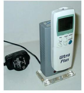
Infrared (IR) remote controls that are supplied with many air conditioners send complex signals compared to television and video remotes, which can make it very awkward to train an ECU.
