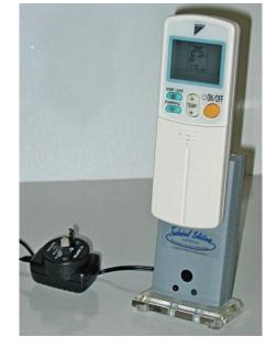
If your air conditioner is not supported by our Universal Air conditioner Interface, we can modify your existing remote control. In this case you must send us your remote and we will then modify it by permanently attaching it to the interface unit. You can usually buy a second remote control from your air conditioner supplier if you can't part with the original for a few days!
