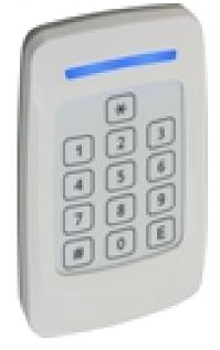
This numeric keypad is supplied as a kit with a controller and installation instructions. It can be used to activate almost any motorised door, gate or lock release. Simple electrical skills are needed to install the kit. Operates from 12-14 Volts which is usually available from the door motor. A seperate power supply is available if needed.
